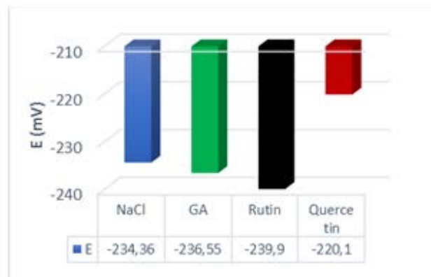
Figure 6. E corr of copper in 3% NaCl solution with the addition of GA, rutin and quercetin in concentration 0.03221 g/l
